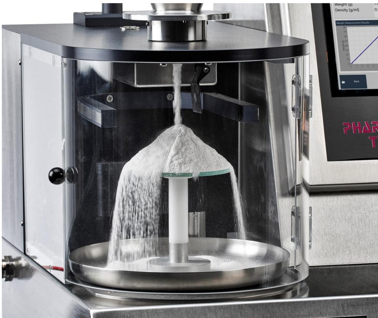
In processes, which rely on powder and / or powder, mix integrity, the need to have the correct powder flow characteristics is paramount. These powder mixes have to be formulated, mixed and certainly transported. Transportation, even over small distances an easily lead to classification of sorts such that “fines” may drop out and alter the particle size distribution and hence the flow characteristics.
