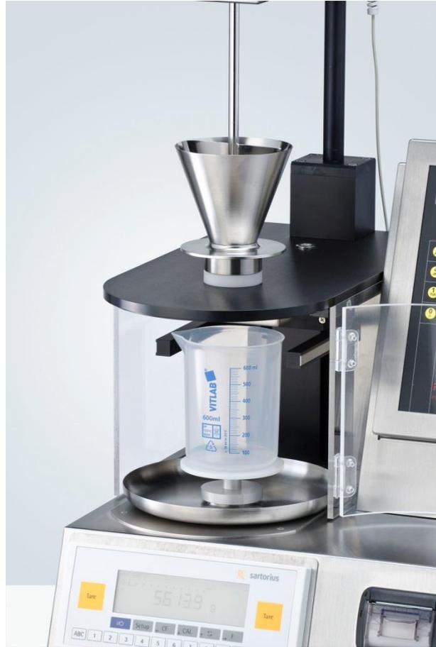
Using the conical stainless steel funnel as described in the current EP/USP monograph and use the changeable nozzles of 10, 15 and 25mm, the cone angle can also be tested. If smaller diameter nozzles are to be used, an adapter ring, which allows the use of pouring nozzles from 4 to 10mm, is available.
