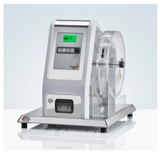
One of the testing criteria for mechanical strength of tablets and cores according to the USP <1216>, EP <2.9.7>, JP <14> and other pharmacopoeia is friability and abrasion testing. During the process of coating, transportation and packing the tablet will lose some amount of weight. To measure this weight loss, the samples are counted and weighed. Then the friability test is performed following the
