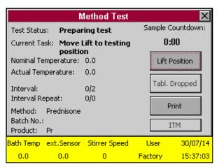
As soon as the test is started, a screen saver can be activated with the most important information displayed in large script, like count-down timer so that this information remains visible even at time when the operator is not standing directly in front of the instrument.
