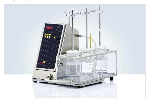
The DIST-3 is used for the manual testing of disintegration times of tablets, capsules and other solid dosage forms. The triple basket DIST-3 version offers the following features:
